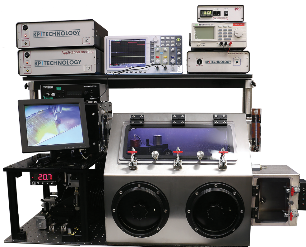
APS04-N2-RH system with ambient pressure photoemission spectroscopy, nitrogen environment and scanning capabilities.
