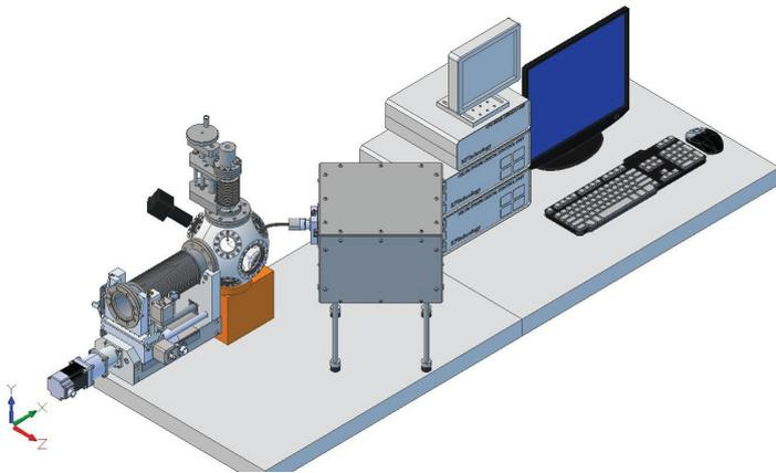
Technical drawing showing full layout of 4 system including light source, camera, control units and PC.
